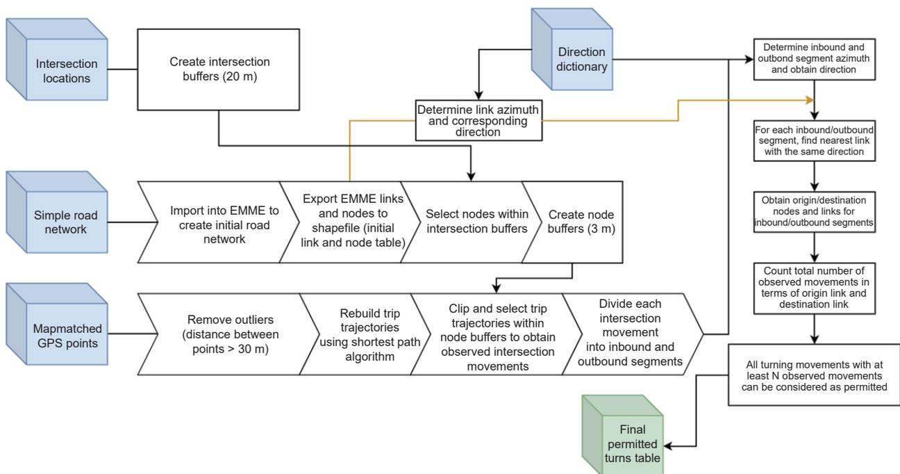
Fig. 5 Turning permission extraction process.
