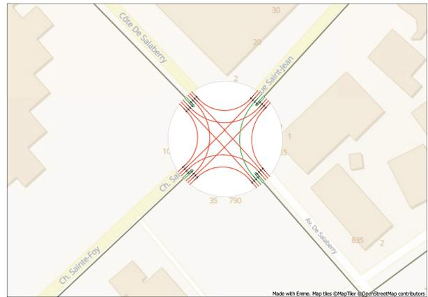
**Fig. 9** Extracted intersection movement permissions (permitted turning movements in red and prohibited movements in green).
